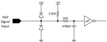
Figure 15: Hall sensor signal input circuit
