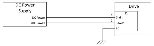
Figure 10: Power supply connection to the drive
