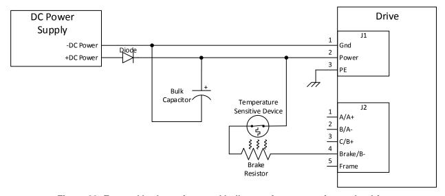
Figure 29: External brake resistor and bulk capacitor connection to the drive
