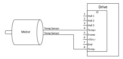
Figure 19: Temperature sensor connection to the drive
