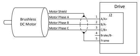
Figure 11: Brushless DC motor connection to the drive
