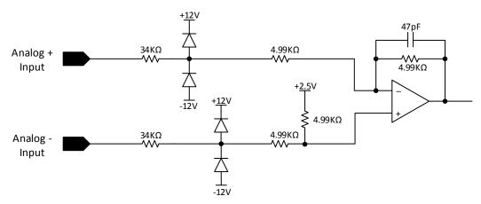
Figure 25: Analog input circuit
