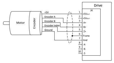
Figure 17: Single-ended encoder connection to the drive
