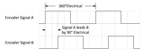
Figure 5: Encoder feedback signal
