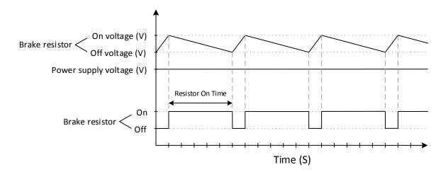
Figure 28: Brake resistor operation graph
