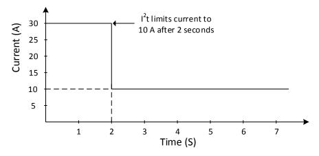
Figure 7: I<sup>2</sup>t algorithm example
