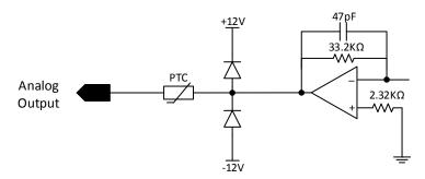
Figure 26: Analog output circuit
