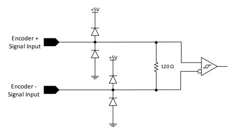
Figure 18: Encoder signal-ended input circuit
