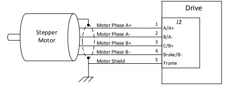
Figure 13: Stepper motor connection to the drive
