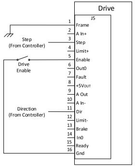
Figure 22: Minimum drive I/O connection needed to operate stepper motor
