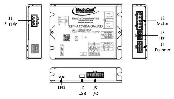
Figure 9: Drive connector layout
