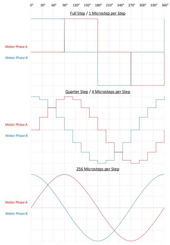
Figure 4: Stepper motor Phase Current Waveform
