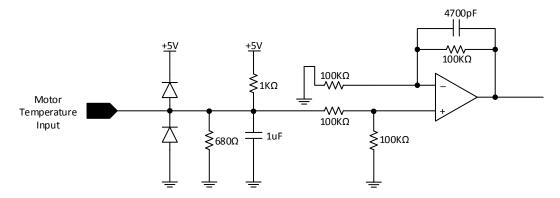
Figure 20: Temperature sensor signal input circuit
